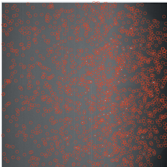
Figure 10 A merged detector image with the 1558 detected spots marked by red rings.
