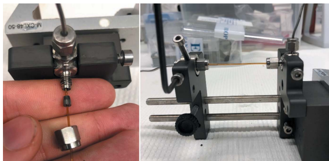
Figure 1 Photographs depicting (left) the assembly of 0.85 mm ( \varnothing OD) fused quartz with polyimide coating, graphite ferrule for 1/16" with 1.0 mm hole and 1/16" Swagelok elbow fitting on the optical rail carrier side, and (right) fastening of the Swagelok fixture in the completed reactor cell.
