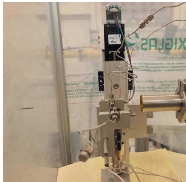
Figure 1 Photographs depicting (left) the assembly of 0.85 mm ( \varnothing OD) fused quartz with polyimide coating, graphite ferrule for 1/16" with 1.0 mm hole and 1/16" Swagelok elbow fitting on the optical rail carrier side, and (right) fastening of the Swagelok fixture in the completed reactor cell.
