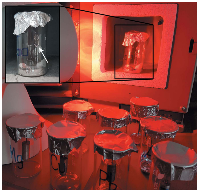
Figure 13 Utilities for puzzle (10): flasks with metal ingots, an infrared lamp, fireproof environment (oven).
