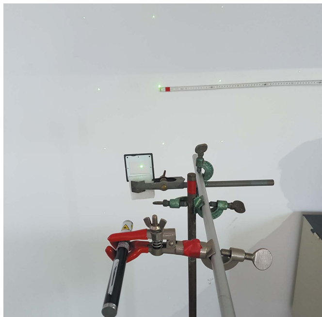
Figure 8 Utilities for puzzle (7): laser pointer, optical grid and a folding yardstick.
