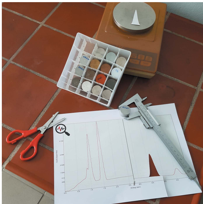
Figure 14 Utilities for puzzles (11) and (12): set of materials with different densities, balance, calliper, part of the characteristic X-ray spectrum, scissors.
