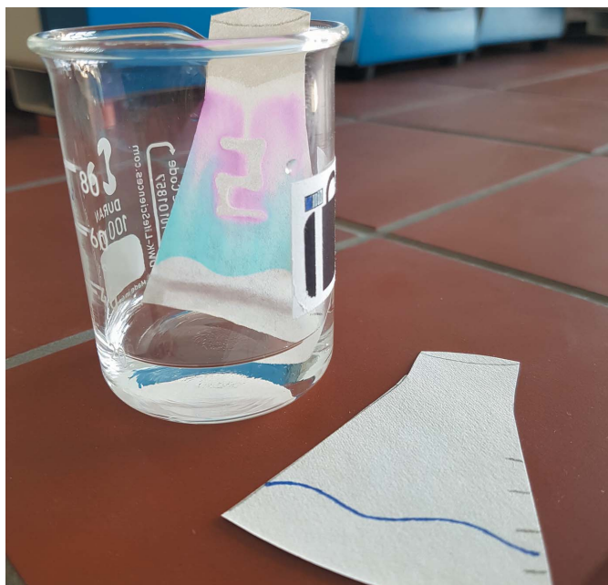
Figure 10 Result of the experiment carried out in puzzle (8). The capillary rise of the water carries the coloured hydrophilic ink towards the top of the filter paper and dyes it. Only the part of the filter paper covered by the transparent hydrophobic ink remains unaffected. The number sought becomes visible.
