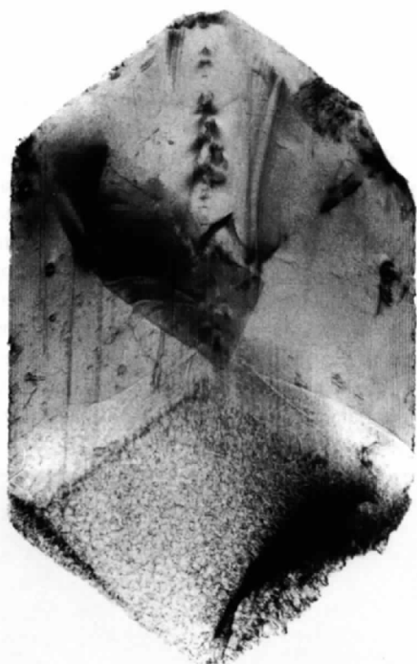
Figure 11 Projection topograph, 004 reflection, \theta_B = 45.95^\circ , \lambda = 0.128 nm. Dominant diffraction contrast comes from cracks, and from polishing striae and other superficial damage. The specimen-to-plate distance being <0.1 that used for the radiograph, Fig. 10, the gross refraction mottle due to Araldite vesicles is here reduced to fine-scale speckle.
