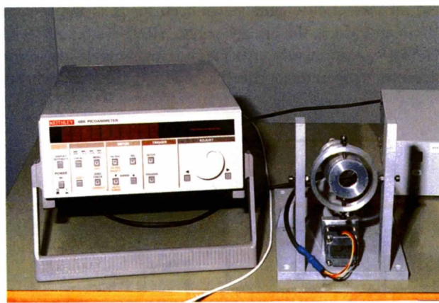
Figure 1 The simple system, based on a gimbal design, used to eliminate the Bragg peaks from the absorption spectra.
