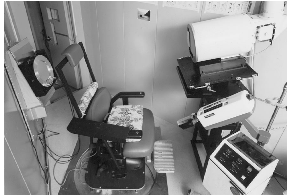
Figure 2 Inside the clinical hutch. A circular X-ray exposure-dose counter on the left-hand side, a special chair for the patient, an X-ray imaging system (II-TV), and an auto-injector for contrast media on the right-hand side can be seen.
