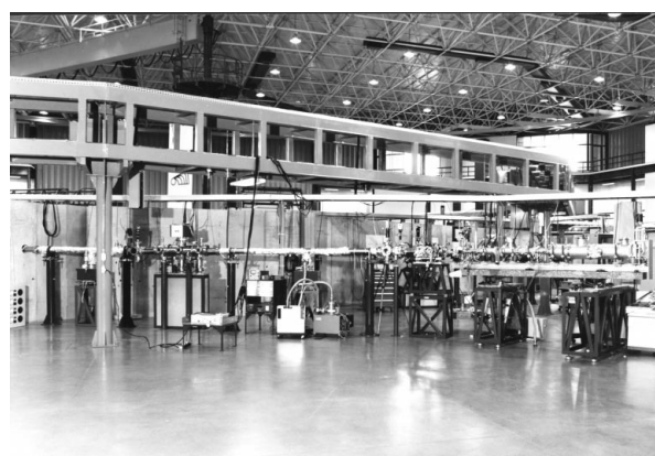
Figure 5 The SAXS beamline. The beamline passes across the shielding on the left. The sequence of optical components is: mirror chamber (for vertical focusing), first four-slit set, monochromator chamber (for monochromatization and horizontal focusing), second four-slit set, guard slit set, sample holder, beamstopper and vertical X-ray position-sensitive detector.
