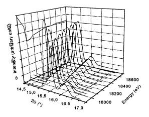
Figure 1 Reflection behaviour of Zr 0002 and Zr 10-11 reflections within an energy range in the vicinity of the Zr-K absorption edge. The projection indicates the development of the Zr 0002 DAFS curve.
