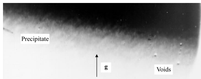
Figure 3 A precipitate and several voids in the 400 transmission topograph of Czochralski silicon.
