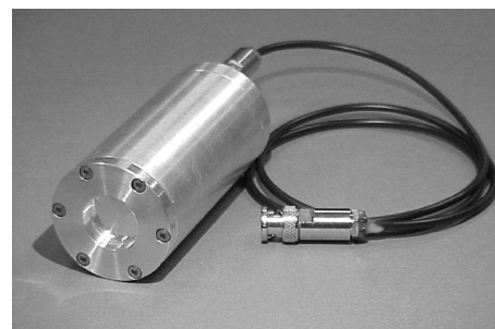
Figure 5 The photodiode-based detector used for measuring DAFS spectra. The dimensions are the same as for common scintillator-based detectors, allowing the use of off-the-shelf detector mounts.
