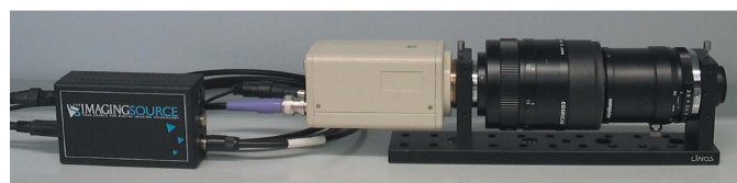
Figure 1 The low-cost detector set-up consisting of (from right to left) scintillator, lens system, CCD camera and frame-grabber.
