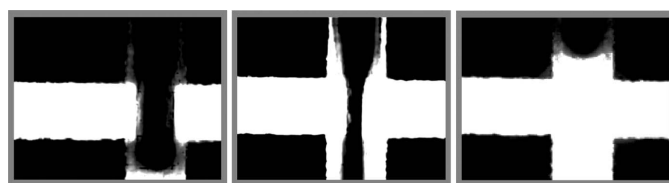
Figure 3 Schematic of the 8CB droplet formation with diffraction patterns observed at three different observation positions along the formation process.
