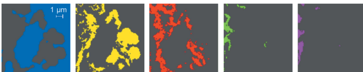
Figure 12 Results of angle distance measure, applied to a stack of images of Chernozem soil taken with the STXM at BESSY II. The distribution maps of the first five clusters are shown. Spatial distribution of the chemical elements identified in Fig. 11.
