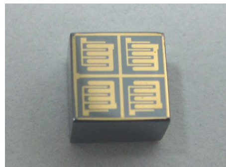
Figure 6 The anode surface of the 2 × 2 CPG-array CdZnTe detector that we designed, with dimensions of 7 mm × 7 mm × 5 mm.
