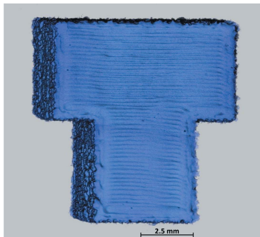
Figure 7 Upper surface of TC showing morphology typical of the final layer of manufacture.
