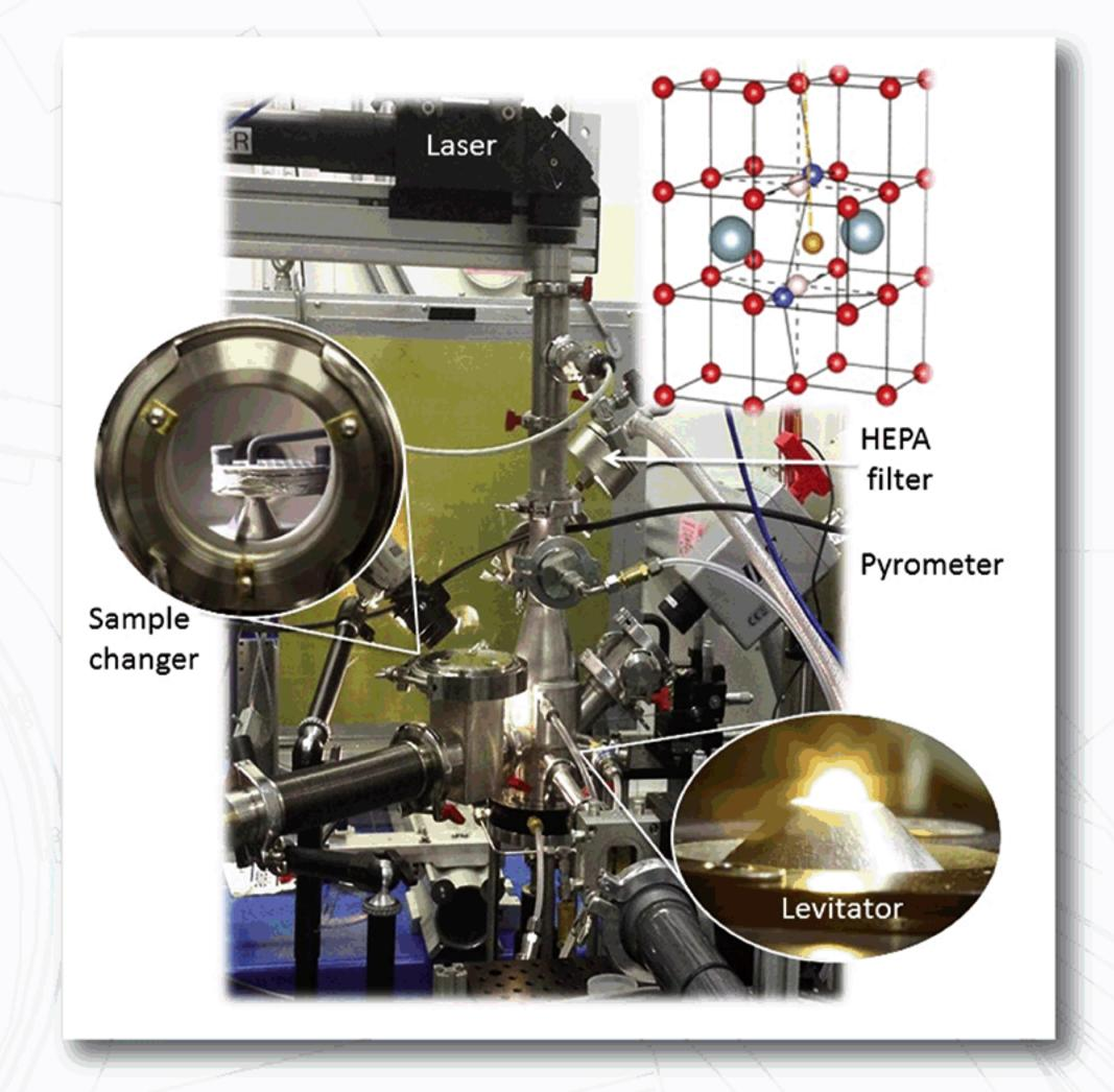
The nuclear material is levitated from below on a gas jet and heated from above by a 400 W CO<sub>2</sub> laser. The scattered x-ray beam is measured with a large, wide-angle, flat-plate area detector. The sample manipulator is operated outside the chamber using a bellows system.
