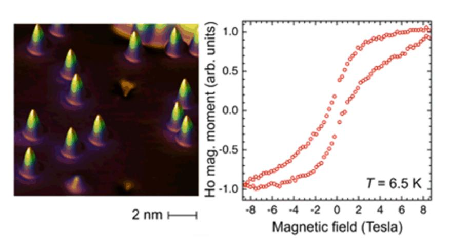
Single holmium atoms adsorbed on few monolayers of magnesium oxide are extraordinarily stable magnets. They retain a significant fraction of their magnetization when the external magnetic field is switched off. This has been shown recently in a study combining x-ray magnetic circular dichroism performed at the Swiss Light Source (SLS) and at the European Synchrotron Radiation Facility (ESRF) as well as scanning tunneling microscopy. The results open perspectives of storing and processing
