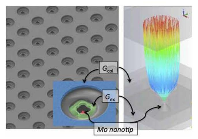
Nanofabricated low emittance field emitter array cathodes were demonstrated for the first time, and successfully applied to observe the low-energy electron diffraction from suspended 1 monolayer graphene. The work has an impact on the future development of compact X-ray free electron lasers, THz/RF vacuum electronic sources, and ultrafast electron imaging and diffraction experiments. Read more:
