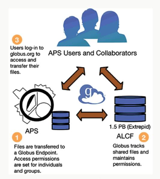
Above: The Extrepid system housed in an ALCF computing center provides 1.5-PB of storage space for the APS. APS users and collaborators can access data using Globus Online. Below: XPCS integrated workflow pipeline depicting data flow from acquisition at APS 8-ID, to the TCS building for computation, and then back to the APS for visualization and interpretation.
