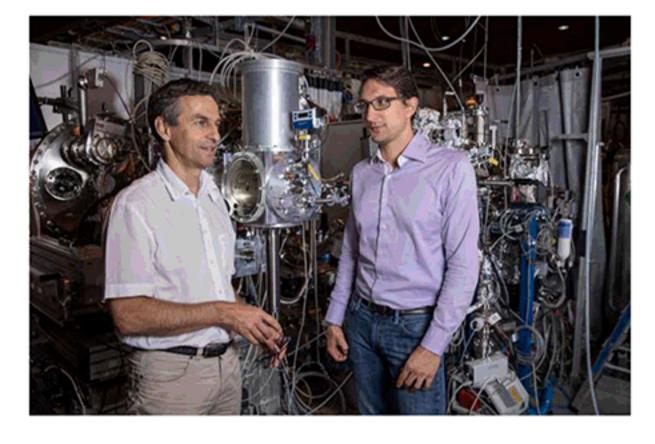
PSI researchers have developed an experimental chamber in which they can recreate atmospheric processes and probe them with unprecedented precision, using X-ray light from the Swiss Light Source SLS. In the initial experiments, they have studied the production of bromine, which plays an essential role in the decomposition of ozone in the lower layers of the atmosphere. In the future, the new experiment chamber will also be available for use by researchers from
