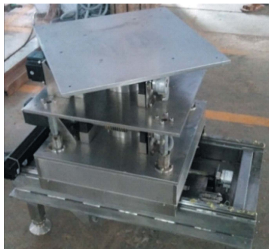
Figure 3 The X - Z - \theta motion stage, which can carry a maximum of 500 kg.
