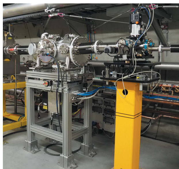
Figure 1 Top: schematic of the setup in the SASE2 tunnel: filter chamber, K-mono, SR-imager. Bottom: photograph of the K-mono and SR-imager in the SASE3 beamline.
