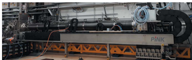
Figure 7 Photograph of the the SAXS configuration with AGIPD located at the maximum distance of \sim 8 m from the sample.
