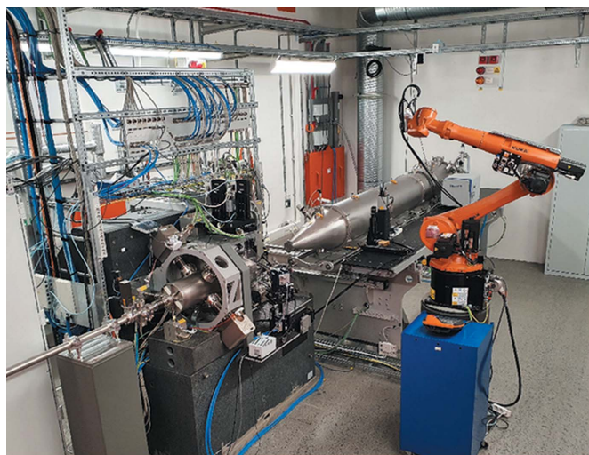
Figure 5 Left: photograph of the diffraction endstation with the detector robot and the vacuum flight tube. Right: top view of the diffraction endstation hutch. A: granite support, B: detector vacuum flight tube, C: breadboard for detectors and equipment, E: KB-optics chamber, F: radiation safety shutter, G: goniometer, H: sample position, K: fluorescence detector, L: Eiger detector, M: Merlin detector, N: Pilatus detector, O: detector robot, P: Crytur detector, Q: chicanes, R: electronics cabinets, S: pumps, chillers etc. V: ventilation exhaust. Ventilation inlet is through the hutch ceiling (not shown).
