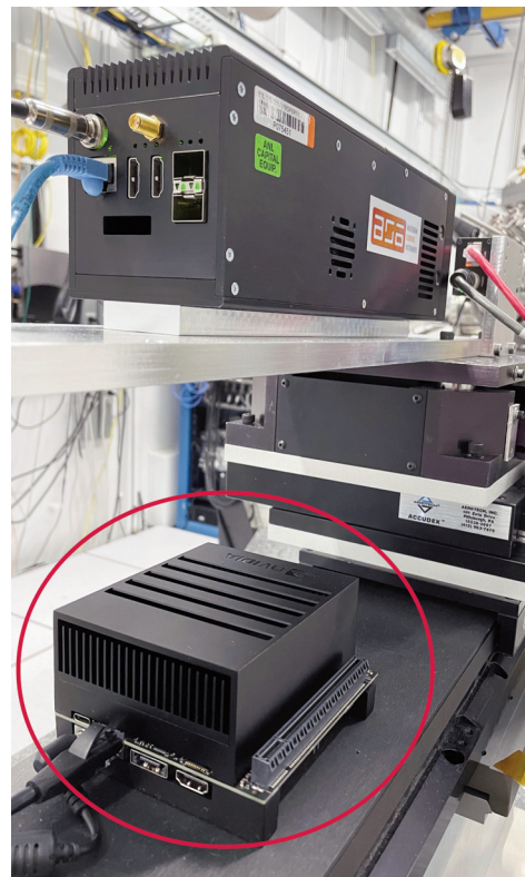
Pictured above is the Jetson edge device (circled) running PtychoNN, which makes live predictions from the detector (top) data stream and sends them to the beamline computer. Photo: Mathew Cherukara (Argonne/Advanced Photon Source)
