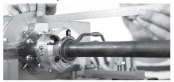
The MAX IV 3 GeV storage ring vacuum system is the first of its kind, with the inner surface of the chambers coated with a non-evaporable getter material. A paper in the Journal of Synchrotron Radiation summarises the results of this unique and successful design choice. Read the full story
