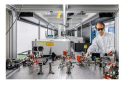
An upgrade at the soft X-ray beamline of the free electron laser SwissFEL will open up new experimental capabilities. Using an external laser system to 'seed' the emission of X-ray photons, and thus imprint well-defined optical properties on the beam, the upgrade gives the Athos beamline unprecedented stability. With this, ultra-fast 'attosecond' timescales that probe the movements of electrons in chemical reactions become possible.
