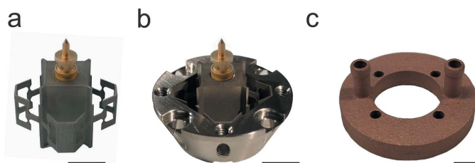
Figure 4 Modifications of the fIOMNI sample holder. (a) An OMNY sample pin inserted into the new pin receptor with flexure structures designed to minimize heat transfer and mechanical stress to the laser interferometer mirror. (b) Receptor mounted in the conical mirror mounting piece. (c) 3D printed water cooler mounted to the back of the laser interferometer mirror. Scale bars: 5 mm.
