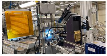
Researchers from Tampere University investigated the effects of deformation speed on the phases that steels might assume during deformation at DanMAX beamline. What they learn could be used to improve the design of the next generation of materials. Read the full story
