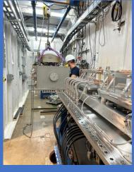
Visual inspection of high-heat-load mirrors at the APS metrology lab (above) and their installation in POLAR's first optical enclosure (left). The G and H experiment stations include nano-focusing K-B mirrors for spot sizes as small as 100 (400) nanometers, respectively.
