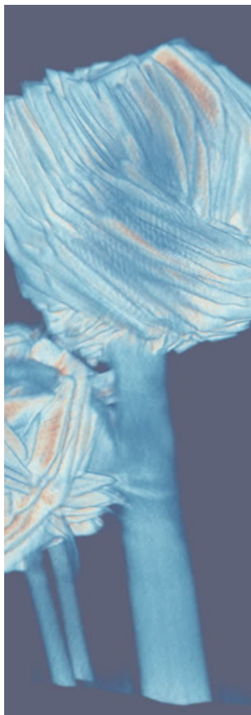
Above: A schematic of the PtychoProbe beamline layout to be constructed at beamline 33-ID of the Advanced Photon Source. Left: An X-ray ptychographic tomography of copper sulfide secondary particles. PtychoProbe will enhance our current capability in both spatial resolution and imaging speed. Image: J. Deng, et. al, Rev. Sci. Instrum. 90, 083701 (2019)
