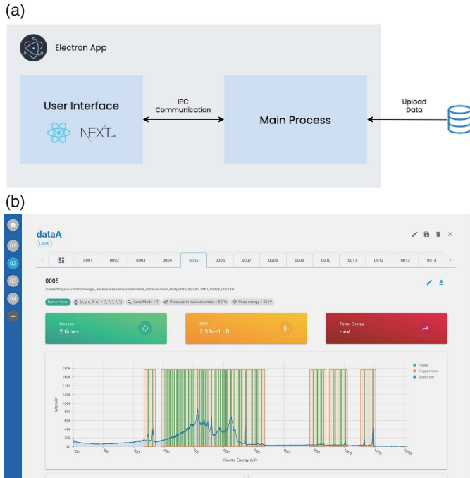
Figure 1 The graphical user interface of synapse . (a) Architecture. (b) User interface.
