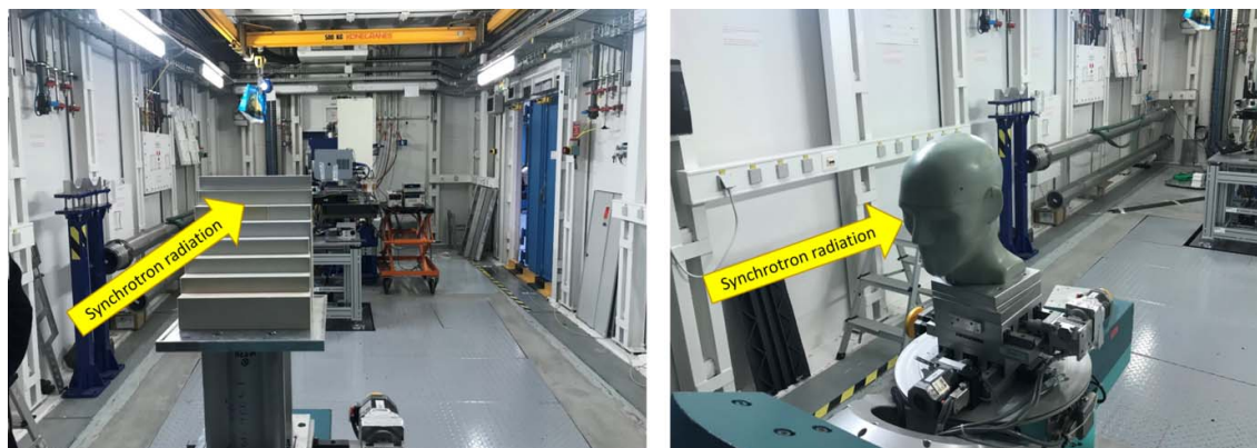
Figure 3 Photographs of the RW3 staircase phantom with thicknesses ranging from 2 to 16 cm (left) and of the human head phantom (right). The detector was positioned 6 m behind the phantoms.
